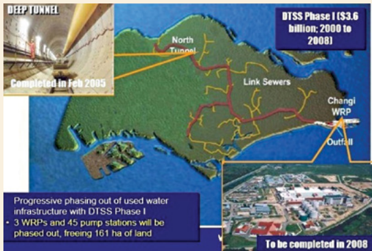
Deep Tunnel Sewer System (DTSS)
